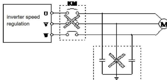
Fig.1-3 Capacitor is not permitted to use at the output side of inverter
