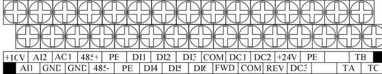
Form 3-7 Control Panel Terminal Arrangement Order Diagram
