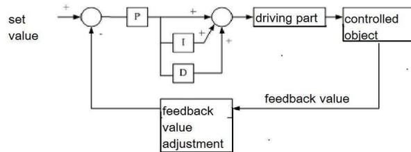
Fig. 6-21 PID system structure
