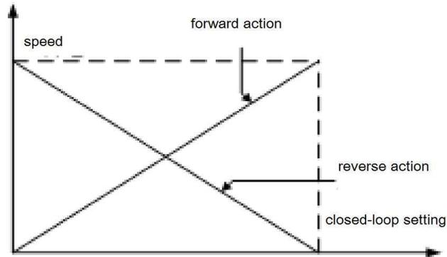
Fig. 6-22 forward/reverse characteristics illustration
