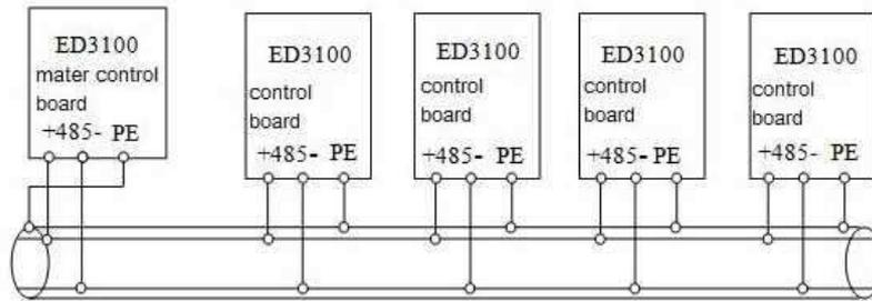
**Form 3-13 Wiring Diagram of the Inverter communication( The Inverter and the Motor should be well grounded)**
