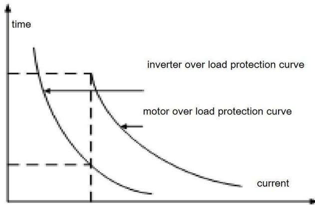
Fig. 6-30 inverter's overload protection and motor's overload protection curve
