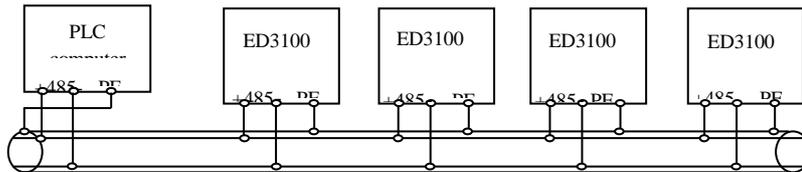
**Form 3-12 Wiring Diagram of communication between PLC and the**
