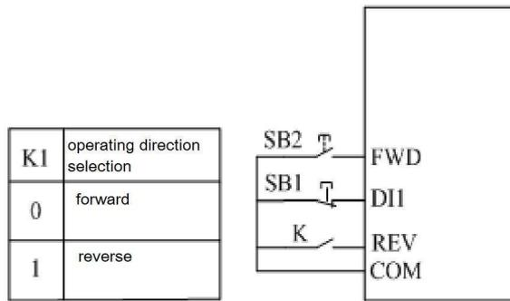
Fig.6-14 3-wire type control mode 2
