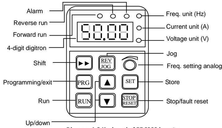
**Diagram 4-2 Keyboard of PR6000 inverter**
