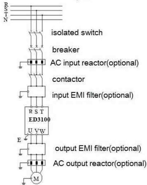
**Fig. 3-4 The connection between inverter and optional components.****3.4.1 Connection between the Inverter and the Accessories.**
