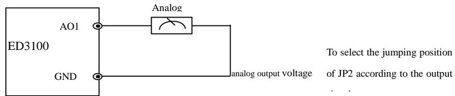
Fig. 3-10 Simulation Output Terminal Wiring
