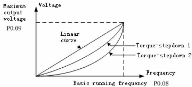
Figure 6-4 Multiple V/F Curve Diagram
