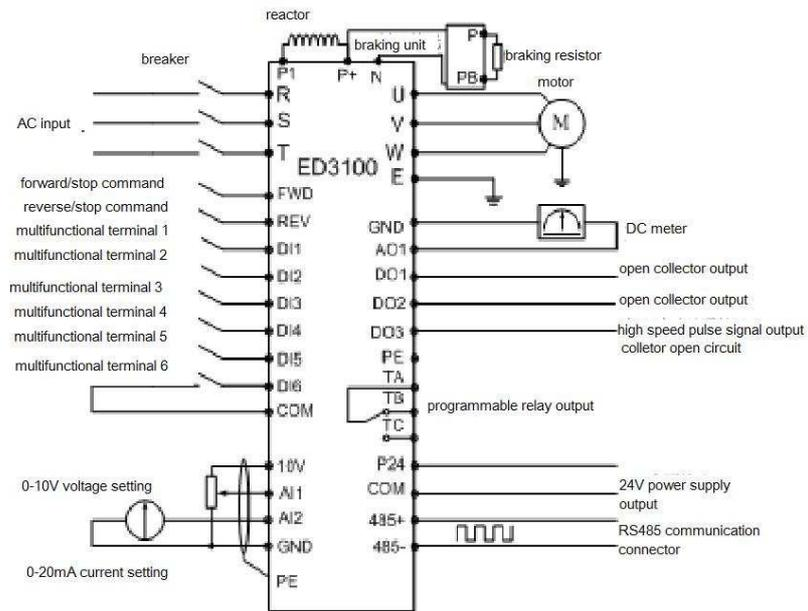
Form3-6 Basic Running Wiring Diagram FIT MODELS: ED3100-4T0220M~
