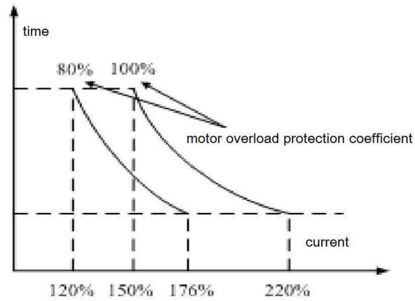
Fig. 6-31 Motor's overload protection efficient setting.
