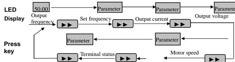
Diagram 4-7 Example of Run status parameter display operating
