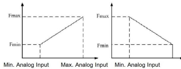
Fig.6-19 The corresponding frequency setting value of Max. and Min. Analog input
