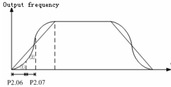
Figure 6-7 S Curve Diagram
