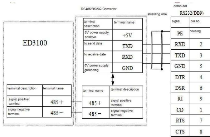
**Form 3-11 RS485—(RS485/232)—RS232 Communication Wiring**
