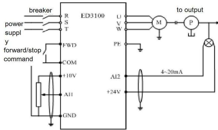
Fig.6-20 analog feedback control system schematic
