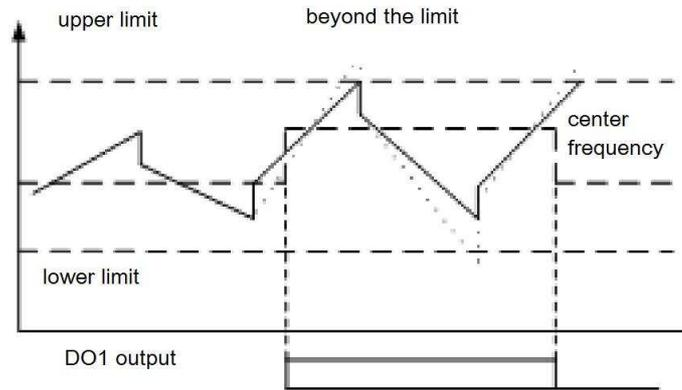
Fig 6-15 transverse operation upper and lower limit schematic
