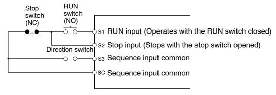
**Note** Set parameter 052 to forward/reverse rotation command 0 for 3-wire sequence input.
