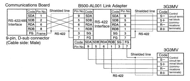
**Note** Turn the terminal resistance of all the Inverters to ON for RS-422 communications. Refer to page 2-18, *Selecting RS-422/485 Termination Resistance* for details.
