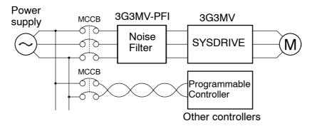
**Note** Use a special-purpose Noise Filter for the SYSDRIVE 3G3MV. A general purpose noise filter will be less effective and may not reduce noise. Please, use the noise filters as explained in Chapter 9-2.
