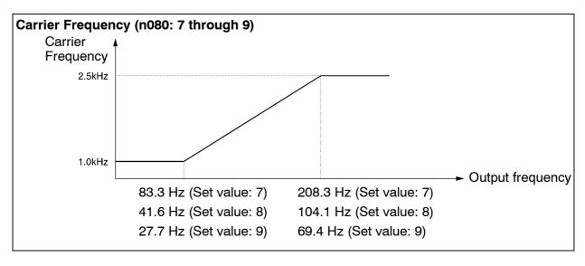
• The Inverter cannot maintain rated output current with the carrier frequency set to a value higher than the default one.
