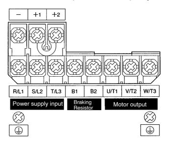
**Note** For single-phase input, connect R/L1 and S/L2.
