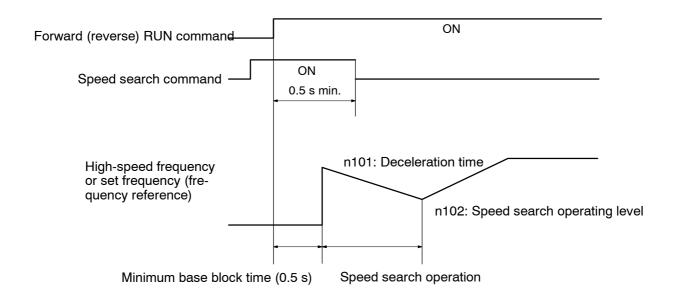
**Note** For 5.5- and 7.5-kW Inverters only, the speed search function can be adjusted by setting parameters n101 (speed search deceleration time) and n102 (speed search operating level). If the speed search cannot be executed properly using the default setting, lengthen the deceleration time or lower the operating level. To reduce the speed search time, check with the application while either shortening the deceleration time or raising the operating level.
