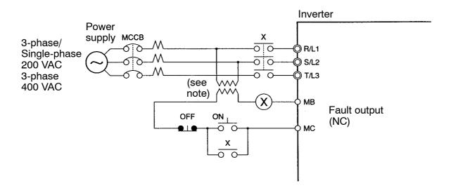
**Note** Use a 400/200 V transformer for a 400-V model.
