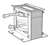
The DC Reactor suppresses harmonic current generated from the Inverter and improves the power factor of the Inverter. The DC Reactor suppresses harmonic current more effectively than the AC Reactor. Furthermore, the DC Reactor can be used in combination with the AC Reactor.
