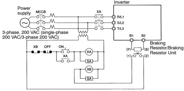
Contact points for thermal trip of Braking Resistor Unit or external thermal relay
