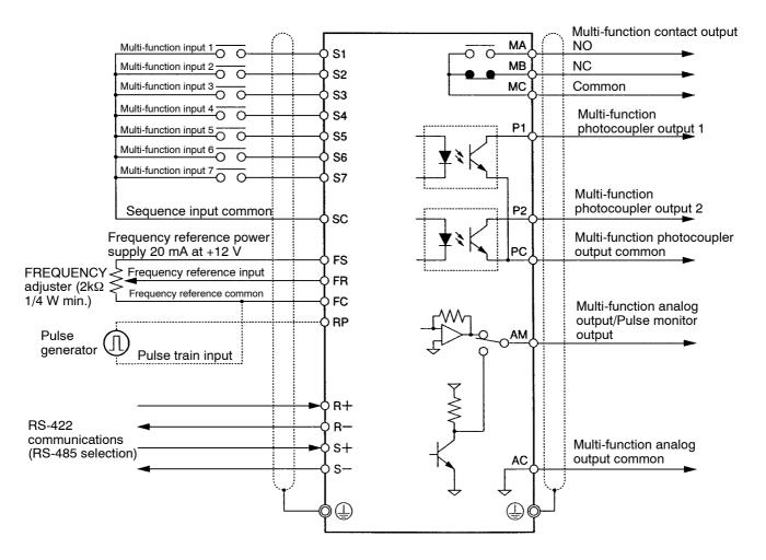
**Note** I/O signals can be connected to a single shielded cable.
