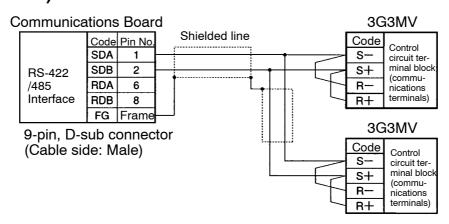
**Note** Be sure to set the terminal resistance of only the Inverter at each end to ON and that any other Inverter to OFF. Refer to page 2-18, *Selecting RS-422/485 Termination Resistance* for details.
