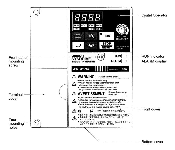
**Note** None of the following 200-V models have a terminal cover or mounting holes. Instead, the front cover is used as a terminal cover and two U-shaped cutouts are provided in place of the mounting holes.
