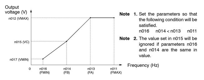
• Set the rated motor frequency as the maximum voltage frequency, and set the rated motor voltage as the maximum voltage.
