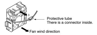
3. Slide the protective tube and remove the internal connector.
