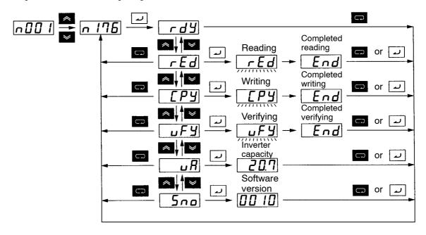
Note The following display is an example of the capacity displayed.
