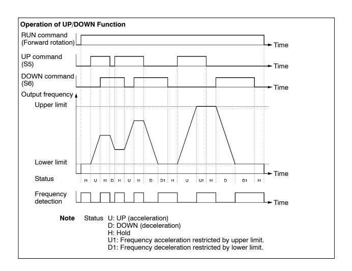
• The following ON/OFF combinations of UP and DOWN commands are possible.
