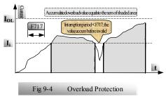
**c.** When sum of shaded area is more than overload protection value, overload protection occurs.
