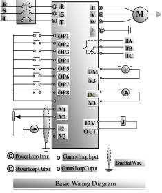
"Three-Line" Connection can fulfill start/stop control by using parameter setting and terminal definition, as indicated in the right Figure. If F200=1, F202=1, start/stop command will be excuted by terminals respectively; F409=6, OP2 is defined as running terminal; F410=7, OP3 is defined as stop terminal. When OP2 or OP3 are connected with CM terminal, it will control inverter's start and stop respectively. Take care that these two terminals cannot be connected to CM at the same time.
