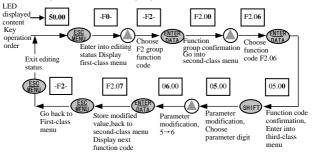
Fig.4-7 example for parameter setting and modification
