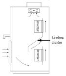
Fig. 3-2 Mounting of multiple inverters
