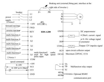
Fig. 3-6 basic wiring diagram
