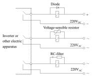
Fig.3-12 Installation demand for electromagnetic on-off device
