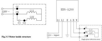
Fig. 3-4 Wiring methods between inverter and motor
