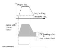
Fig.6-8 Dec stop+DC braking
