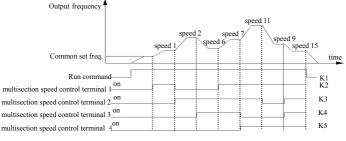
Fig.6-25 multi-step speed run
