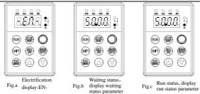
Fig.4-3 inverter electrification, waiting, run status display
