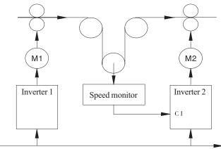
Set the master frequency to other inverters by keypad or computer serial port Figure 5.21
