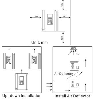
Notice: If the inverter is installed in the (power) cabinet, install fans for heat dissipation.
