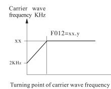
When inverter running frequency is larger than the turning point of carrier wave frequency, the carrier wave frequency setting value will become the maximum value. On the contrary, according to the running frequency the carrier wave frequency will auto tuning between the maximum value and minimum value.
