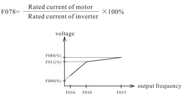
Figure 4.2 V/F curve diagram
