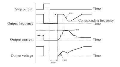
Figure 5.6 time diagram of tracing speed
