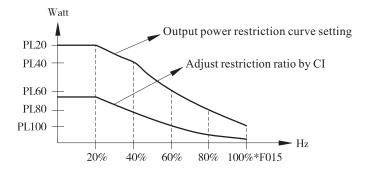
Figure 5.5 diagram of output power restriction curve
